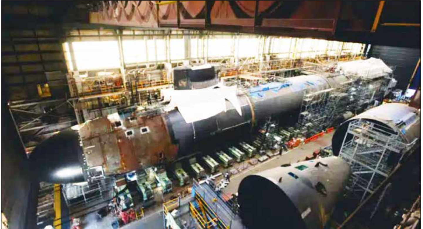
Pressure hull of the USS Massachusetts (SSN-798). (Huntington Ingalls photo.)
